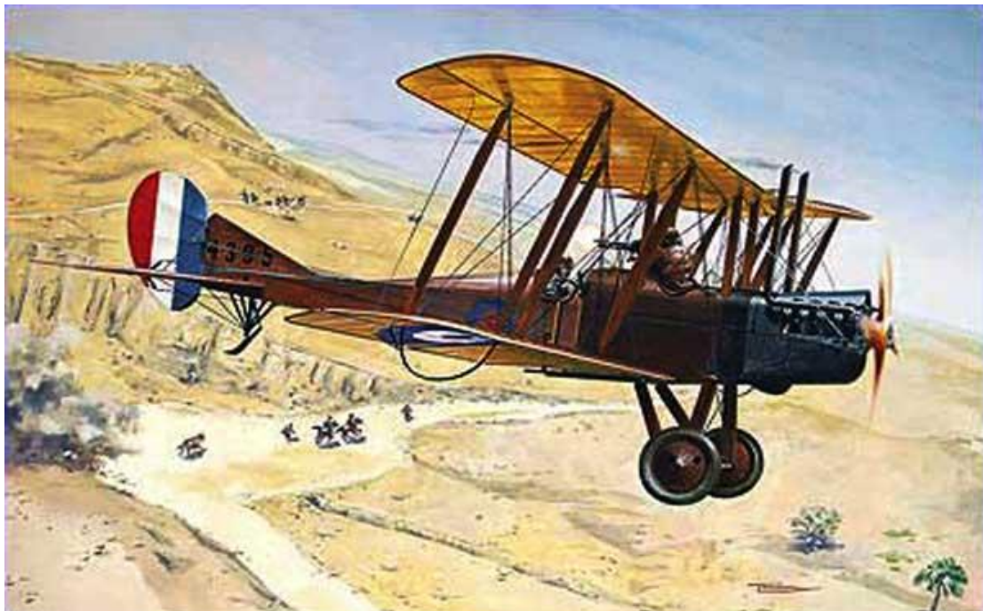
Figure 9: The earlier B.E.2 reconnaissance plane. With the observer in the front, no effective machine-gun arrangement was possible
