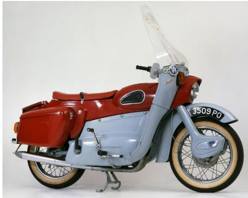
Figure 8: Ariel Leader twin-cylinder, two-stroke motor cycle
